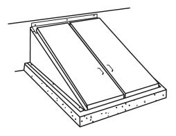
Adjust frame and doors by moving them from side to side until you find the point at which the doors will open and close without binding.
