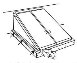
Use prepunched holes in sides and sill as a guide, drill holes onto the foundation 13/4" deep using a 1/4" masonry bit. Install plastic rawl plugs and fasten with 11/2" screws until snug. Check door alignment again. Over tightening will cause misalignment.
