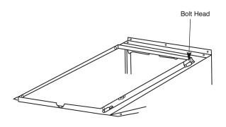
Use 1/4" bolts and nuts from hardware package. Bolt heads must face the outside of the door frame. Nuts on the inside. **NOTE:** The sill bends toward the house.
