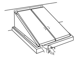
To avoid leakage caulk around frame and promptly paint the door using alkyd base outdoor metal enamel paint. **NOTE:** Do not cement over flanges.
