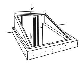
Align frame on foundation and attach **only** at center hole in header.
