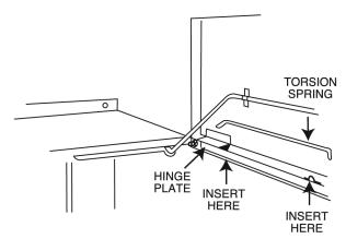
Insert torsion springs by sliding the spring **under** the hinge plate. Point faces downward and inserts into spring clip. If new cement, allow to set before inserting springs. Models CD-1 and CD-2 have 2 torsion springs. Model CD-3 has 4 torsion springs.
