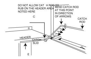
Install catch rods into catch slides. Adjust rods by bending them slightly. Do not allow them to rub on the header.
