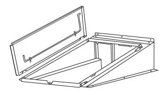
Align the door with the upper and lower pins. Slide door bushing onto door pins.
